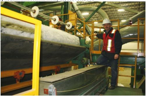
Dan Madlung, chief executive of BioComposites Group, at the firm's new plant in Drayton Valley which produces engineered fibre mats of wood fibre and polyester (white fluff) that is used by auto parts firms to make door panels and trim. The pilot plant will use a variety of materials, and also plans to make erosion control mats.
