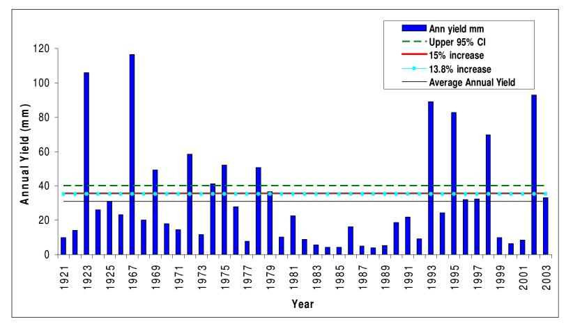
Figure 7 Annual water yield for Beaver Creek near Brocket (1921-2003), average annual water yield, ECA-AB simulated increase in annual water yield with respect to an "informal "15%" rule and upper 95% confidence interval. Simulated 13.8% increase in water yield was less than "15%", and not significantly different from the average annual yield.
