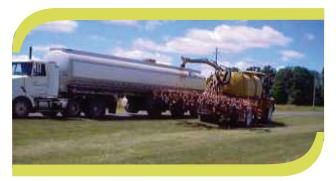
Tankers can be used to move manure to the field, allowing application equipment to continually apply manure.
