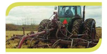
The use of pipeline or dragline manure application systems can significantly reduce the transportation costs associated with liquid manure management.
