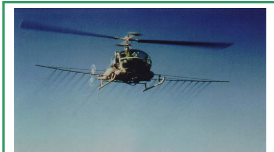
Figure 98. Aerial Herbicide Application
