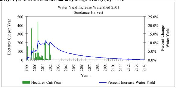
Figure 8 Simulated increases in annual water yield for watershed 2502, Sundance Industries FMA. Watershed size 81.2 km<sup>2</sup>, % harvested 17.2%, max water yield increase 6.3%, max% ECA 8%, hydrologic recovery 5 years. Arrow indicates time of hydrologic recovery ( $\Delta Q \sim 5\%$ ).
