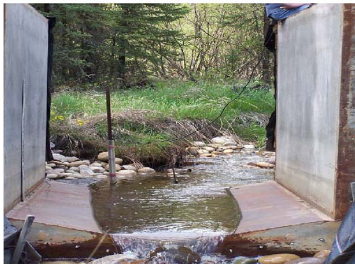
Workshop field tour participants viewed a FORWARD water monitoring station. Automated water samplers are programmed to collect samples at regular intervals, thus enabling the collection of storm water runoff. Data loggers record stage height and water temperature.
