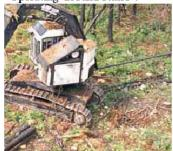
Tracks minimize the impact of machinery on soils by distributing the weight across a greater surface area.
