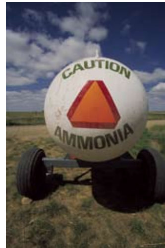
Anhydrous ammonia tank — Courtesy of AAFRD
