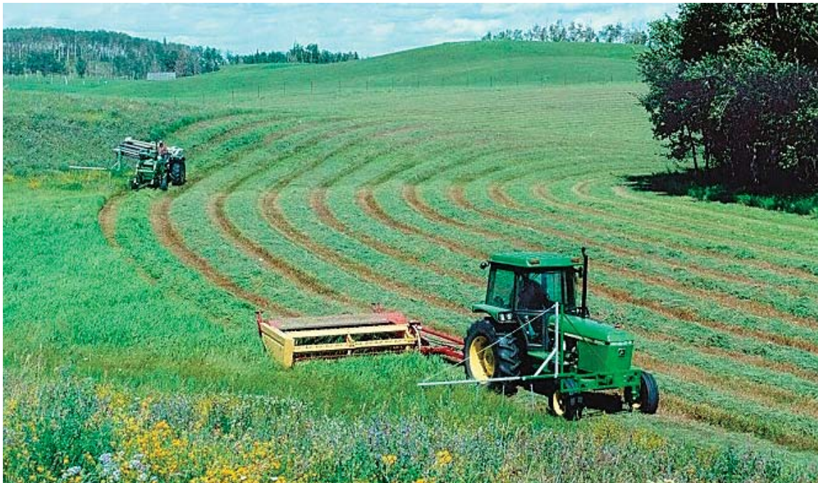
➔ Flushing bar mounted on a tractor.
