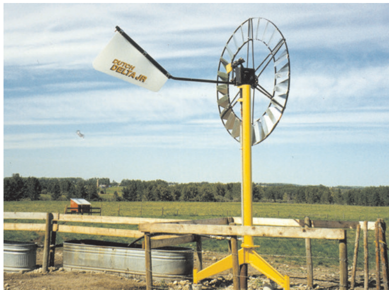
Figure 5-17 Wind-powered Pumping System
