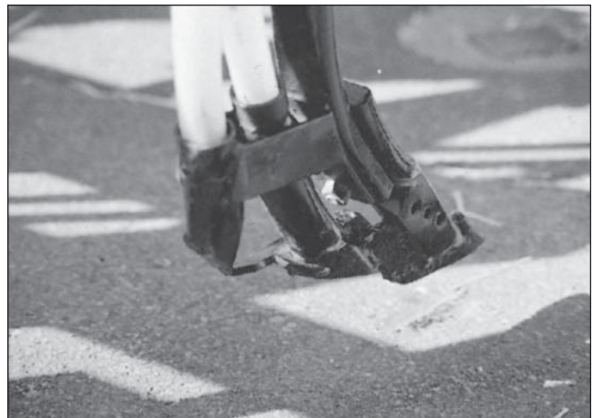
Figure 4. Double shoot single side band opener
