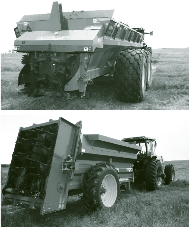
Figure 4.5.4 Examples of Common Solid Manure Application Equipment
