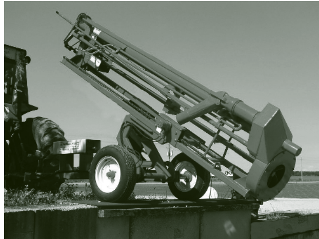
Figure 4.5.2 Example of a pump used to agitate liquid manure prior to application.
