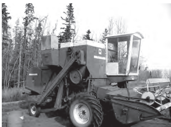
Figure 22. Combine used for mechanical harvest of seed cones
