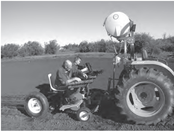
Figure 10. Transplanting equipment for planting echinacea
