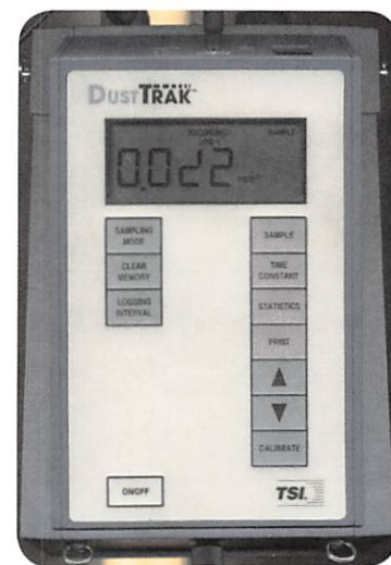
Figure 9. Dust data logger
