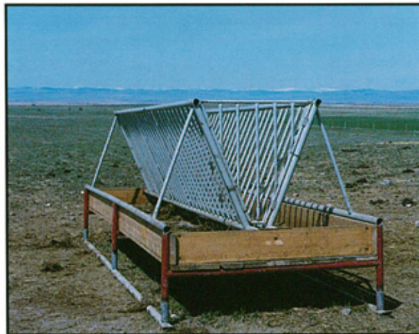
Figure 38. Commercial feeder with bottom pans
